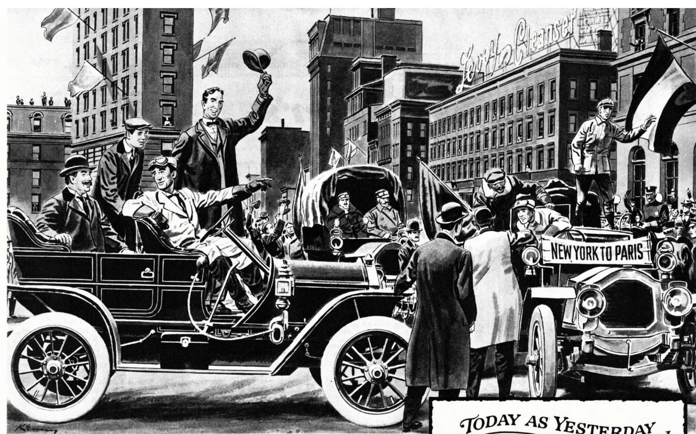
1908 OAKLAND was the ancestor of the present-day Pontiac. This touring model had a two-cylinder, 20-h.p. engine and claimed 20 to 40 per cent less weight than any car in its class.
